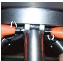
3. Tighten screws with 5 mm. keys
