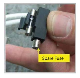
The fuse and a spare are located inside AC power socket
