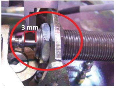
**Caution!** To prevent damage due to bottoming out of the damper during operation, ensure that there is approximately 3 mm. clearance between the damper head and the body when the damper arm is fully pushed in. Use loctide on damper mounting nuts to prevent loosening by vibration if clearance adjustment is performed.
