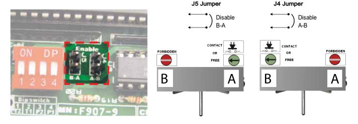
• **Tripod Turnstiles:** Time out and mode settings of the turnstile are selected by the dip switch located on the control board as explained below.
