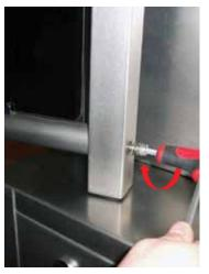
3. Tighten bottom fixing screw
