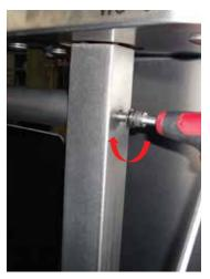
2. Tighten top fixing screw
